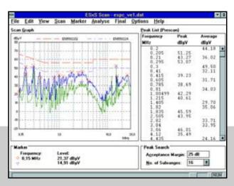
R&S ESxS-K1 is especially designed to provide users of all R&S ESS, R&S ESHS, R&S ESVS and R&S ESCS 30 receivers with a cost-effective Windows based remotecontrol display and storage solution.
